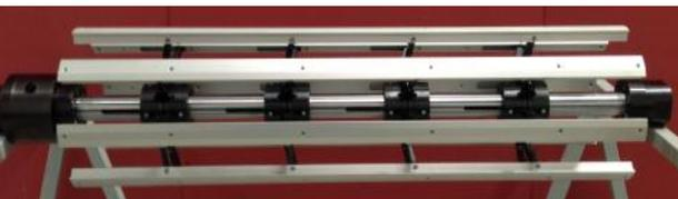
Expanding mandrels (left) are available for all types of foil and strip, including copper, aluminum and paper, Custom built to your requirements, these are optimised for speed and ease of operation in the workplace.
