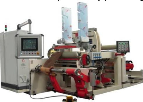
Electronic sensors detect the position of the foil and paper edges, to ensure precise alignment throughout the winding process.
