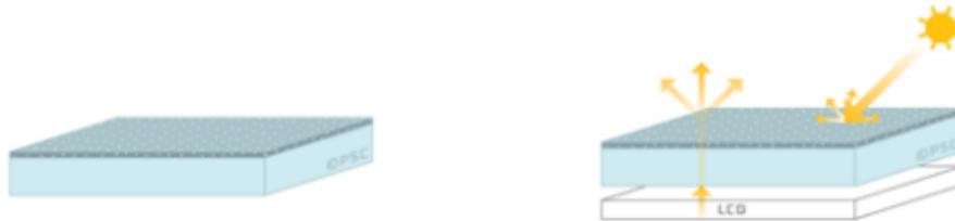
The Hard Mat surface treatment is a UV-cured, non-glare hard coating characterised by extremely good physical and chemical properties. PSC offers Hard Mat surface treatments, which are suitable for both interior and exterior use.
