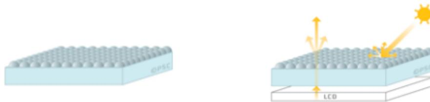
When two plane surfaces are placed against each other, an undesirable phenomenon (Newton rings) can occur. However, Fine Mat acts as a spacer, creating sufficient distance between the surfaces to prevent this occurrence.
