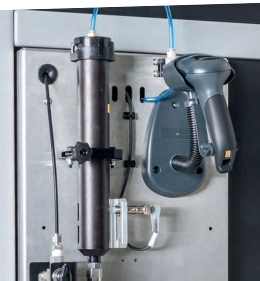
Consistently traceability via handheld bar code scanner and the material identification are logged!
