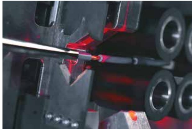
▲ Laser sensors For cable detection
